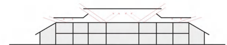
Low Ceiling subdivision - minimal cooling load but with little daylight penetration
